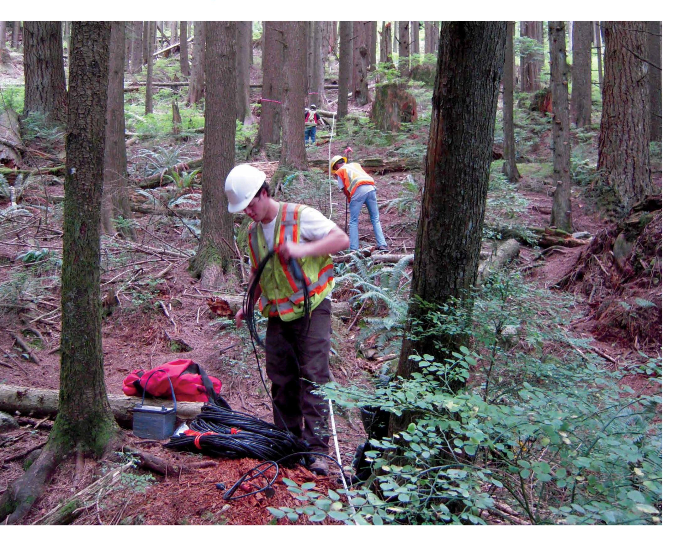
Electric Resistance Tomography (ERT) is geophysical technique that images sub-surface areas by measuring resistivity; the opposite of conductivity. Measurements can either be made with an alternating current or direct current.
