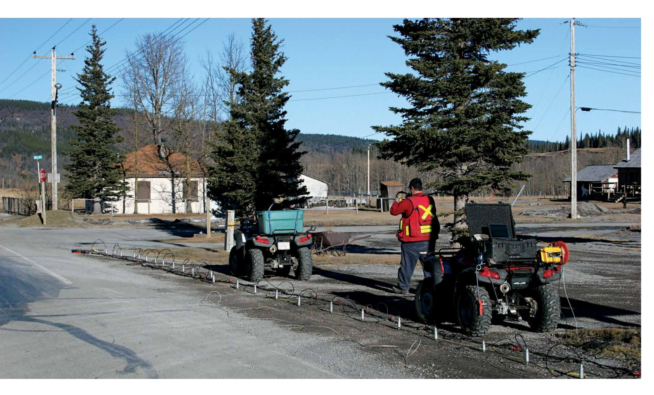
MASW is a seismic exploration method that has been used since the 1990s to evaluate ground stiffness. It measures the velocity of seismic surface waves generated from various sources (such as a sledge hammer).
