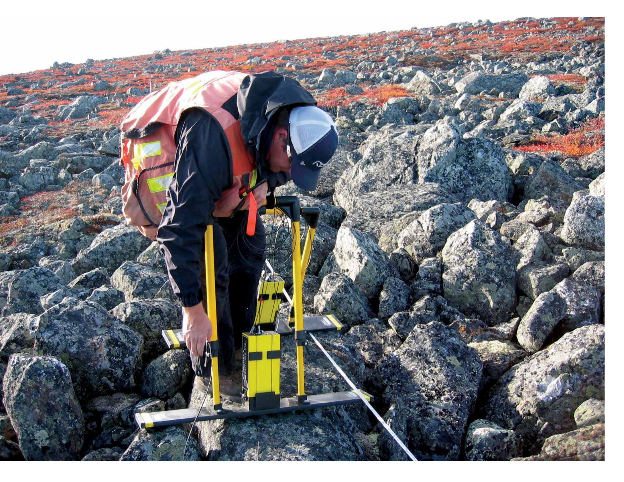
Ground penetrating radar (GPR) equipment uses radio waves to probe subsurface objects. It is flexible and doesn't necessarily need to follow a straight line.
