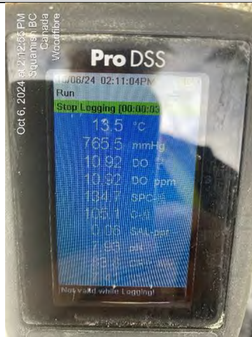
Photo 9: YSI readings in East Creek during discharge
